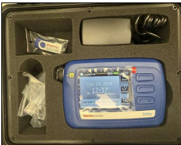
A handheld spectrometer designed to detect substances like fentanyl on surfaces.
